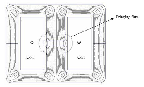
The fringing flux reduces the reluctance of the gap due to the fact that the effective area of the gap is larger than the cross area  $A_g$  of the core face forming the gap. In the case of the above gapped pair of E cores,  $A_g$  is just of the center post. It is then required to introduce a compensation factor, called fringing factor,  $F(\ge 1)$  so as to properly depict the realized reluctance factor  $r_g$  of the air gap by rewritting (7) as the following equation:
