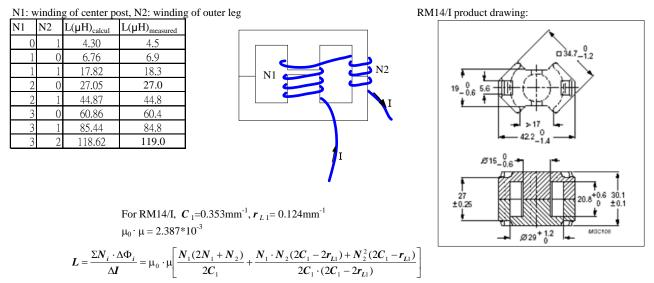
The good fit of the calculation result to the measured data leads to the conclusion that the methodology of magnetic circuit analogy to electric circuit adopted to solve the general inductance equation (6) is workable and effective. It should be noted that winding  $N_1$  and  $N_2$  in (6) could be input as negative integer to represent the opposite pole direction of the concerned magnetomotive force in the magnetic circuit.
