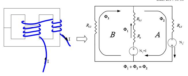
**The** above winding structure leads to unbalanced magnetic flux distribution in the symmetric core set. By analogy to electric circuit, the magnetic circuit can be formed to get the flux solutions for each magnetic path by using Kirchhoff's laws. We can get the flux equation first:
