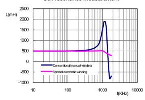
The special automatic winding on the ring core shows better EMI suppression performance
