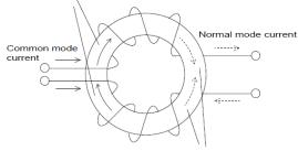
Magnetic flux caused by differential mode current cancels each other, and impedance is not produced.
