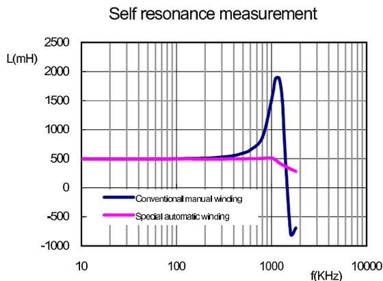
The special automatic winding on the ring core shows better EMI suppression performance
